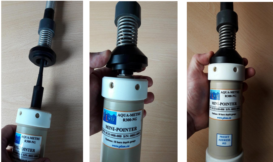
Mini-Pointer R300-NG, simple hydrophone installation
