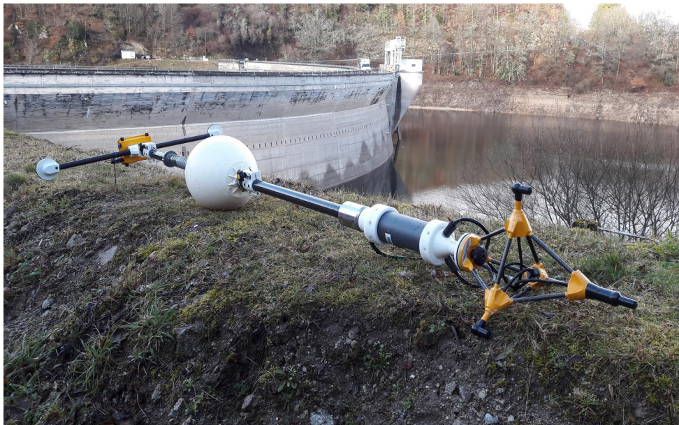
RTKDuo buoy assembled, ready for mooring
