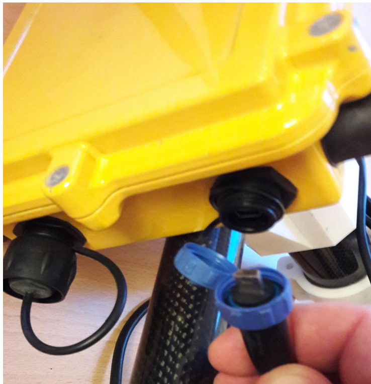
Sensor Section of the RTKDuo buoy, USB mini-AB connector for firmware upgrade
