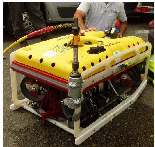
Mini-Pointer R300-NG on ROV FALCON SEAEYE
