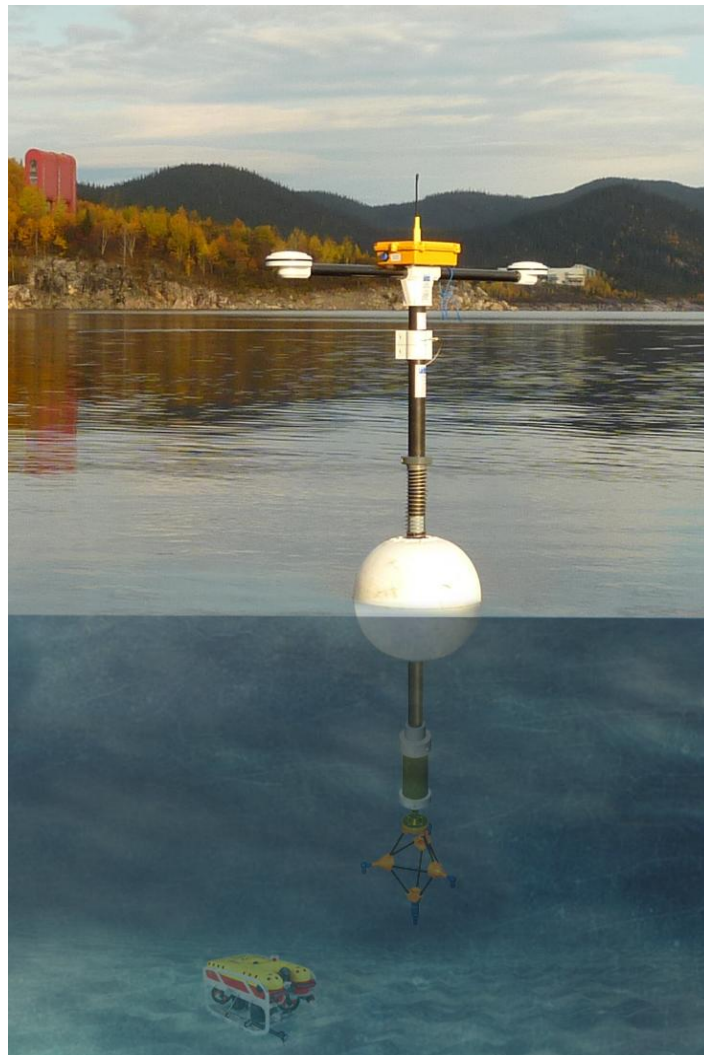
RTKDuo buoy for ROV georeferenced Positionning
