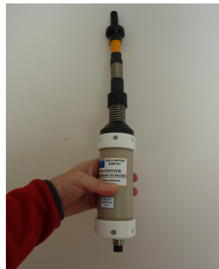
MiniPointer AQUA-METRE R300-NG (alone, right; installed on a survey ROV, left)
