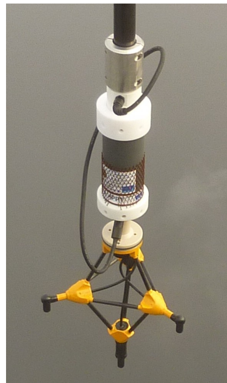
AQUA-METRE R300-NG unit attached to the RTKDuo buoy:
