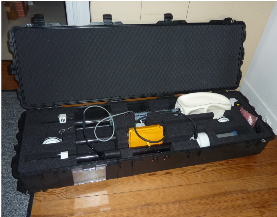
RTKDuo Buoy and Survey Interface in PELICASE 1770
