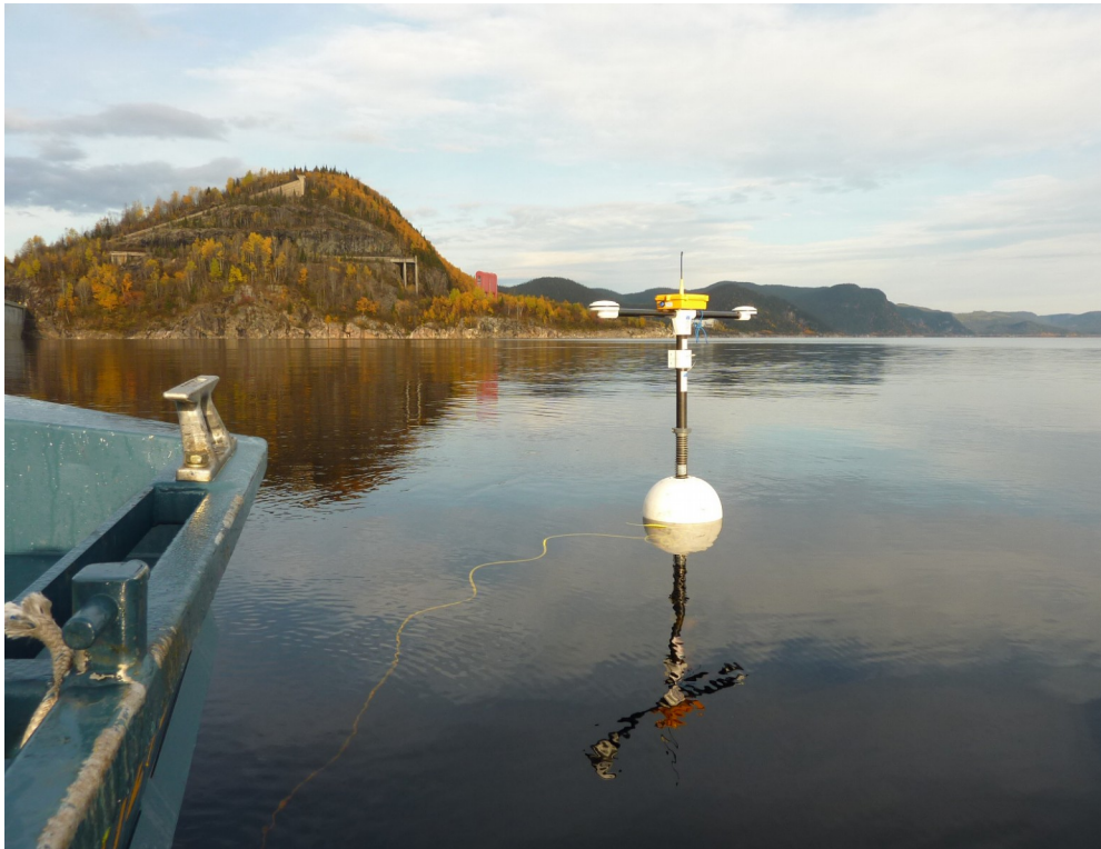
RTKDuo Buoy at Manic5 (Daniel Johnson) dam (QC, Canada)
